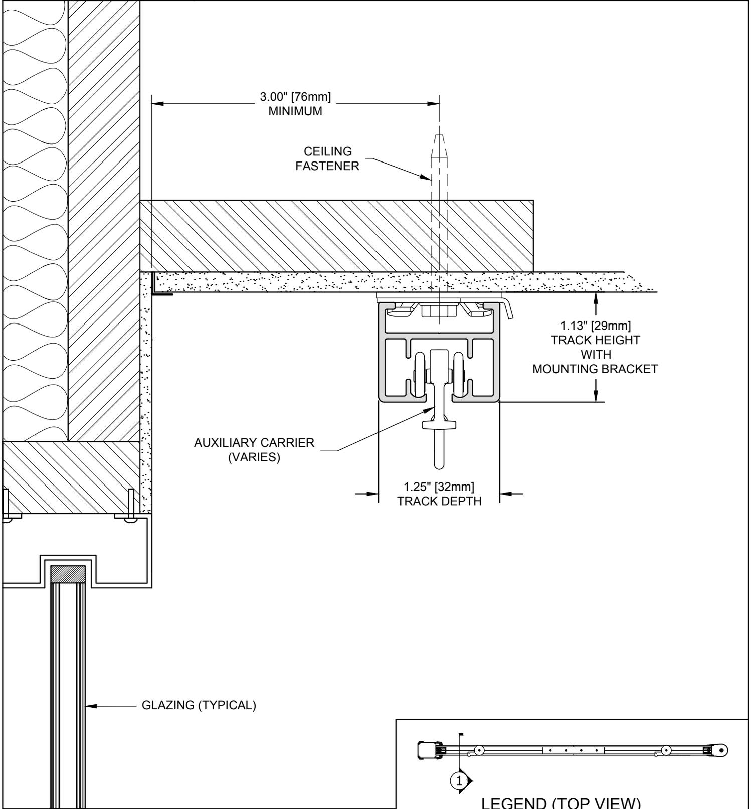
DRAPERY TRACKS INSTALLED AS PROVIDED BY FACTORY PER THIS DRAWING WILL HAVE ALL NECESSARY CLEARANCES FOR PROPER OPERATION OF TYPICAL FABRIC PANELS. IT IS THE RESPONSIBILITY OF THE INSTALLER TO ENSURE PROPER CLEARANCES ARE MAINTAINED BASED ON ACTUAL FABRIC PANEL SELECTION.
